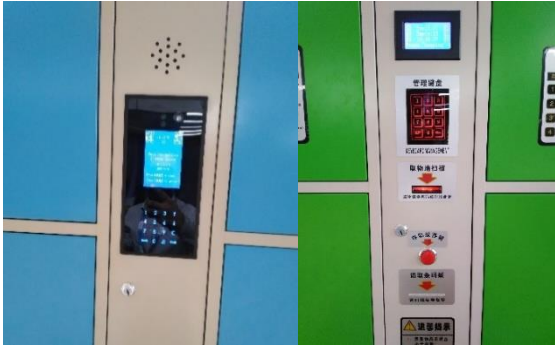
Finger print-based, password protected and Face recognition locker system for students
