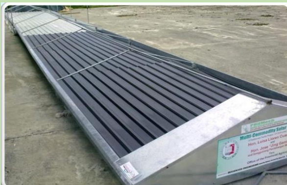
Energy Efficient Multi-commodity Solar Dryer used in Food Engineering Lab with no power and gas requirement
