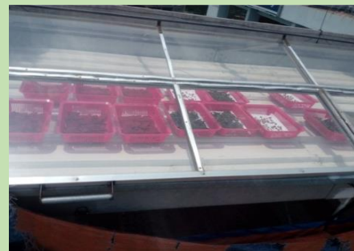
Energy Efficient Multi-commodity Solar Dryer used in Food Engineering Lab with no power and gas requirement
